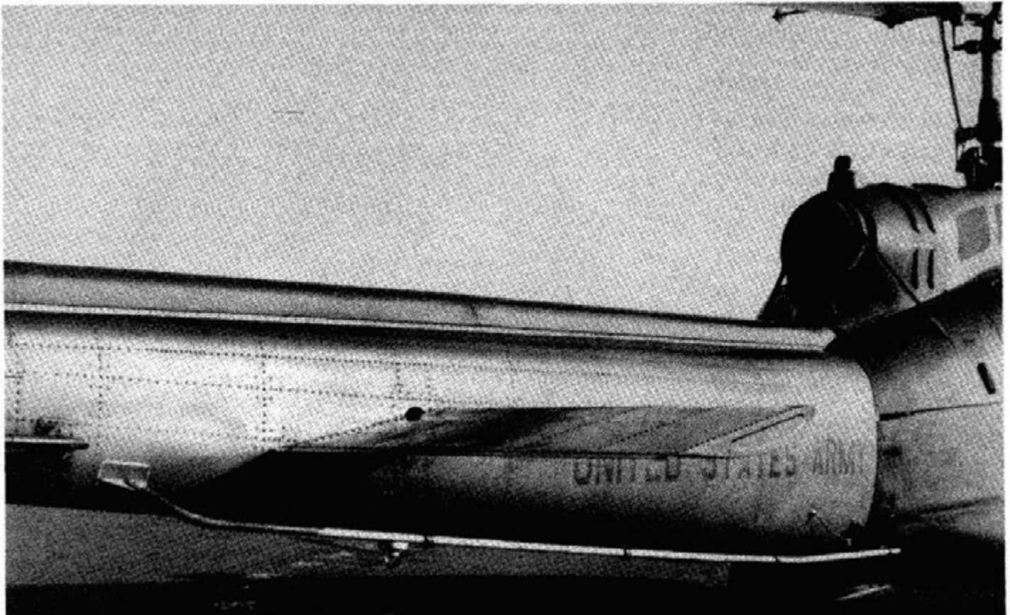
Figure 2. Series AV-600 NVIS antenna installed on Army UH-1
